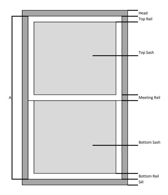
A = Window height for sash balance measurement
