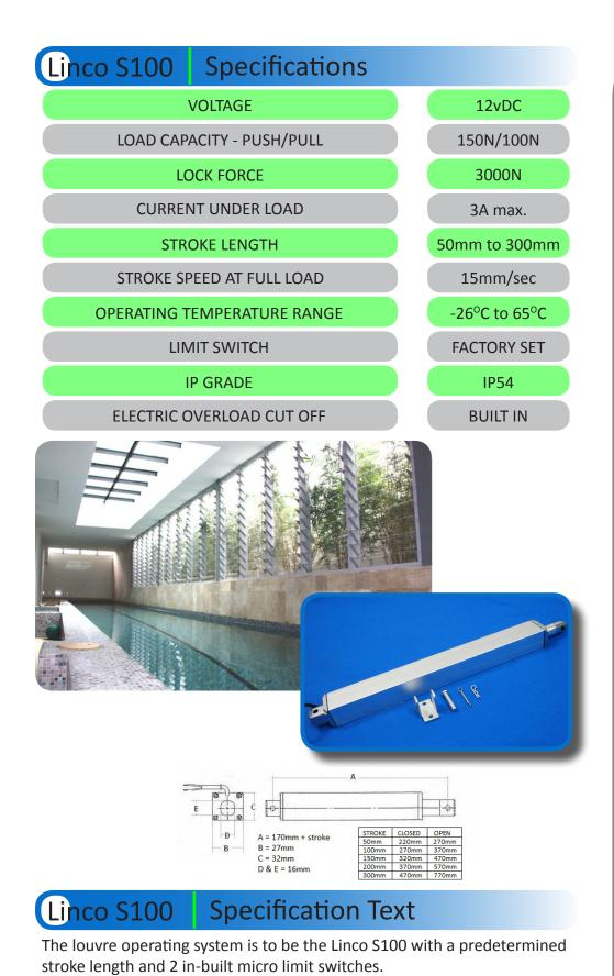
Actuators are to have sintered brass gear drives and be capable of
